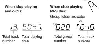
• Total playing time does not appear when MP3 disc is loaded.
